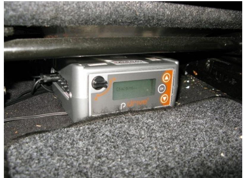
Data logger (pdrive)- under seat
